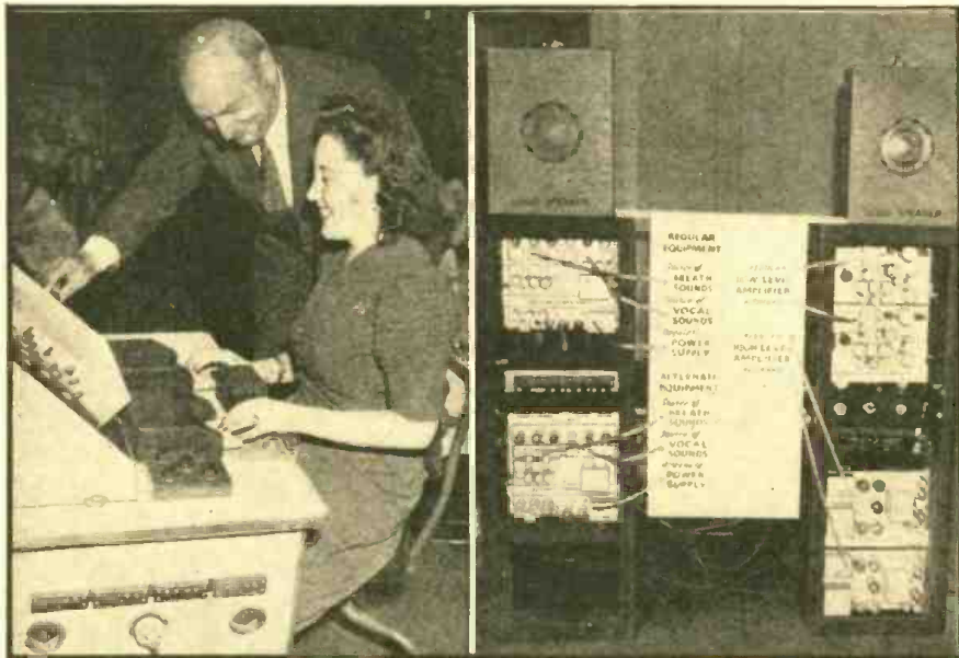
Photo at left shows Voder or synthetic speech control keyboard being operated by Miss Anna Mae Swenson, while Dr. Perrine looks on. Right-hand photo shows close-up of amplifiers and loudspeakers used in Voder demonstrations.
